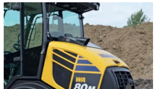
Standard heated rear window and a newly designed, low-profile exhaust pipe ensure improved rear visibility (to ISO 5006).
